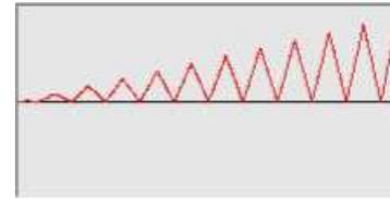
**Sawtooth:** Mod F2 with F1 (AM SSB,  $F2 = 11xF1$ ).
