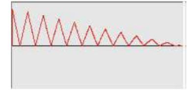
**Inverse sawtooth:** Mod F2 with F1 (AM SSB,  $F2 = 11xF1$ ).
