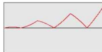
**Sawtooth:** Mod F2 with F1 (AM SSB,  $F2 = 3xF1$ ).
